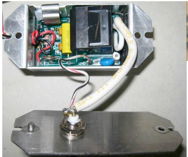
A simple double male BNC will connect the power supply to the ampoule holder in a very compact, light weight package (see picture). 12V for the power supply comes from your system of choice (in my case, from a remote operated switch system).
