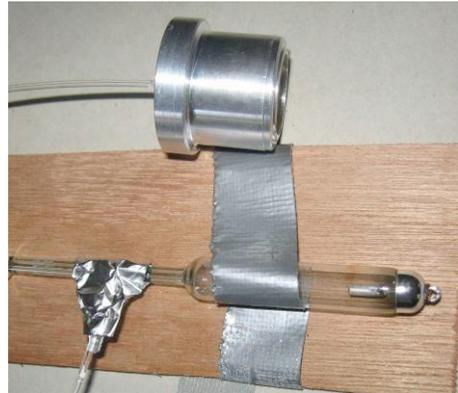
An alternative to the standard discharge tube was to use a small (0.5in x2in long) ampoule containing the gas of interest (these are apparently sold mostly to people who wish to collect samples of the elements). These can be obtained at low cost (approx. \$25 each). They have no electrodes; however, external wires or contacts close to the ends of the ampoule, energized by 2-5KVAC, will excite the tube to glow. The challenge is then the physical and electrical design.
